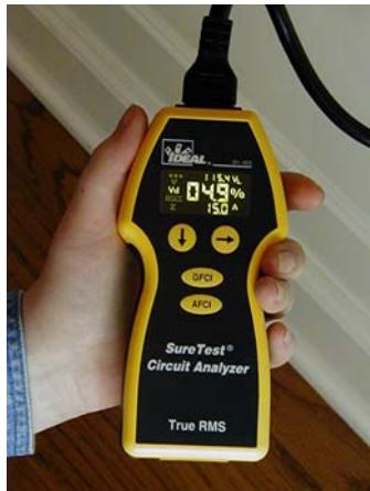
*Voltage drop at a 12, 15, or 20 ampere load can be easily taken by simply plugging the SureTest® into a receptacle and performing the Voltage drop test.*
