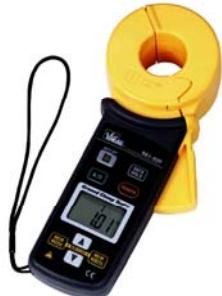
*A ground resistance clamp meter enables electricians to measure the resistance of the ground electrode in a fraction of the time required using the traditional three-point fall of potential test.*
